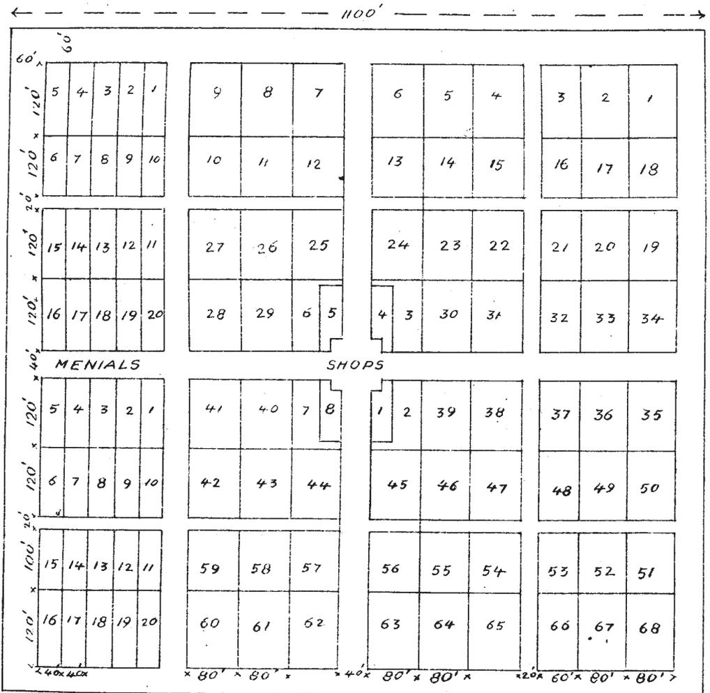
Figure 2.4. Typical canal-colony village layout plan for use in the Jhang and Bhowana irrigation tracts, circa 1900. From Government of Punjab, Gazetteer of the Chenab Colony, 1904 (1905) (Lahore: Sang-e-Meel, 1996), n.p.
